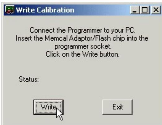
Click on the 'Write' button to begin programming the Flash chip with your calibration. The Status line on this screen will show the status of the programming process. Once the programming is complete the Status line will show 'Write Successful'
