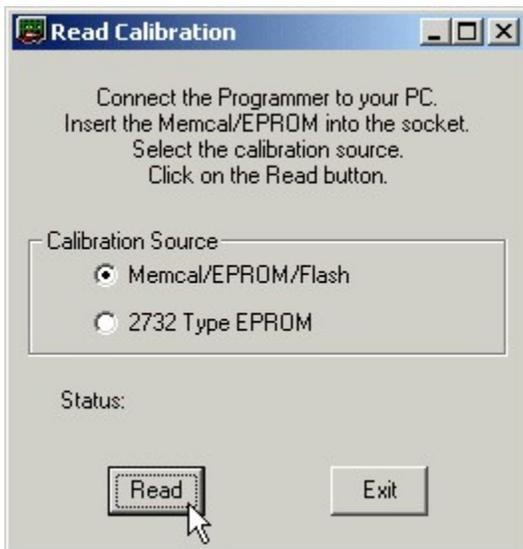
Leave the 'Memcal/EPROM/Flash' calibration source selected and click the 'Read' button. The Tuner program will read the calibration information from the EPROM and load it into the Tuner program. When this process is complete The Status on the Read Calibration screen will show 'Calibration Loaded'
