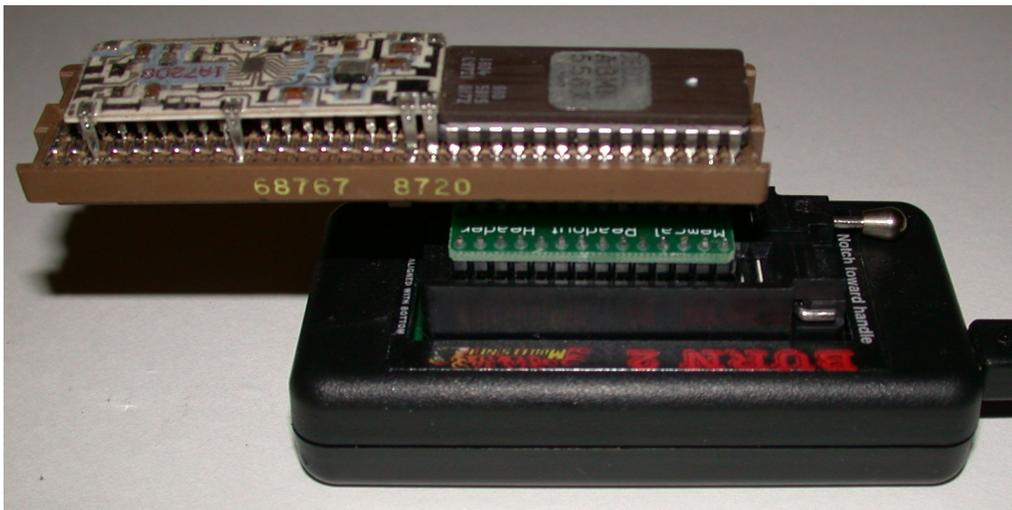
To read the calibration from the EPROM click on the Read Calibration button
