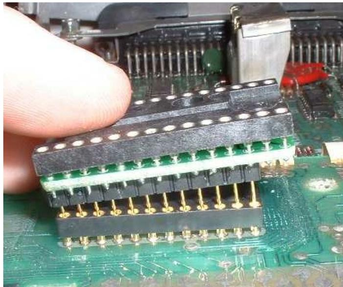
Insert the Flash chip into the G2 adapter verifying that all the pins on the Flash chip are correctly inserted into the socket on the adapter. The notch in the Flash chip must face in the same direction as the notch in the socket.
