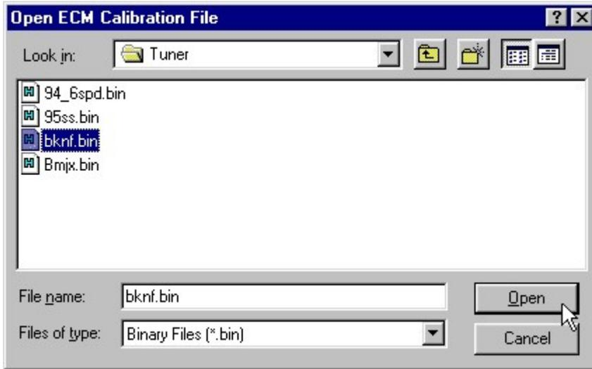
When you select a calibration file and click on the 'Open' button, the program will verify that it is a valid calibration file and that the correct ECM Definition File has been selected. If an incorrect ECM Definition File has been selected an error message will be displayed. If possible, the program will indicate which ECM Definition File is required for the selected calibration.
