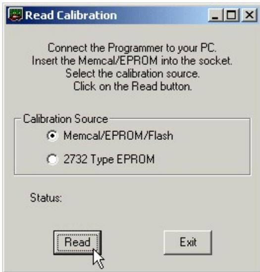
Now click on the '2732 Type EPROM' calibration source and click the 'Read' button. The Tuner program will read the calibration information from the EPROM and load it into the Tuner program. When this process is complete The Status on the Read Calibration screen will show 'Calibration Loaded'
