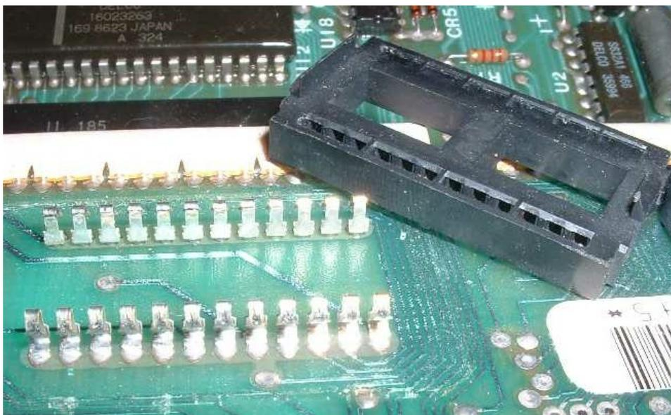
Unsolder and remove all the pins from the PROM carrier socket and clean out the holes in the circuit board with a solder sucker.
