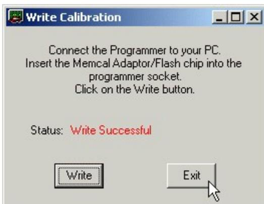
The Flash chip is now programmed and ready for installation in the ECM. Click on the 'Exit' button to close the Write Calibration screen.
