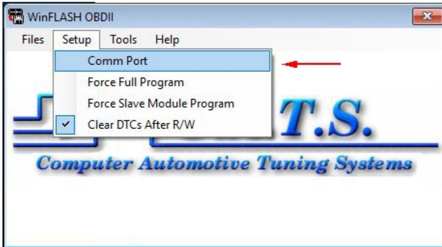
10. On the Comm Port Selection screen click on down arrow to the right of the 'COM Port Number' box and select the COM port number that was assigned to the ALDL cable (it should be shown as 'Available') and then click on the 'OK' button.
